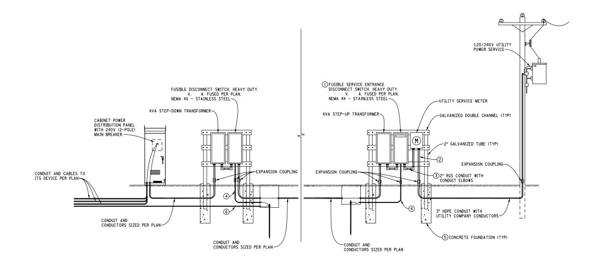
① NEMA 4X SERVICE ENTRANCE RATED DISCONNECT ENCLOSURE. FUSE SIZES PER PAY ITEM AND SPECIAL PROVISION FOR POWER SERVICE. PROVIDE ONE PADLOCK FOR EACH ENCLOSURE. PADLOCK SHALL BE IN ACCORDANCE WITH THE SPECIAL PROVISIONS. PROVIDE AND ATTACH LABEL WITH SITE ADDRESS TO OUTSIDE OF ENCLOSURE.
